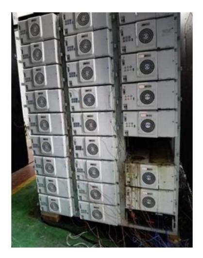
This picture was taken as part of a special fire test that all batteries must undergo and pass, known as UL9540A testing. In this test, the batteries are burned in a lab to verify what types of gases are produced, and to see if the system is designed to contain the fire.
